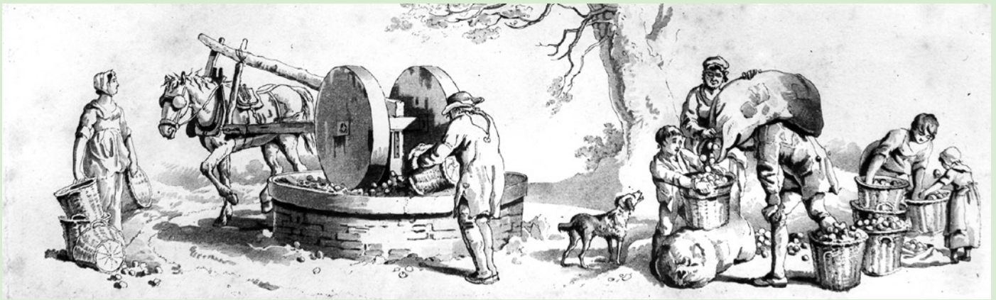
From William Henry Pyne's book 'Microcosm of London', 1808-11, scanned from the book in the Museum of Cider's archives; a horse-mill is being used to bruise cider apples.
